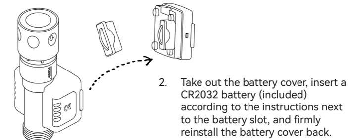
2. Take out the battery cover, insert a CR2032 battery (included) according to the instructions next to the battery slot, and firmly reinstall the battery cover back.
