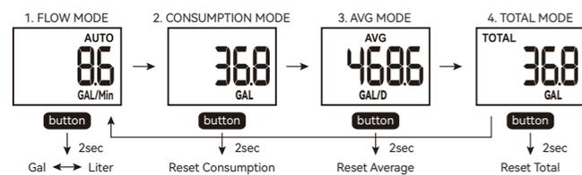
**Press the button briefly:** The display switches to the next display mode.
