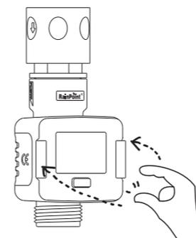
1. Hold the handles on both sides and pull out the display. Or Hold one handle, then push the other side from the back to take out the display.
